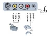
With the 📵 key, select the channel Side. For a monophonic device, connect the audio signal to the AUDIO L input. Use the 🖘 key to reproduce the sound on the left and right speakers of the TV set.
